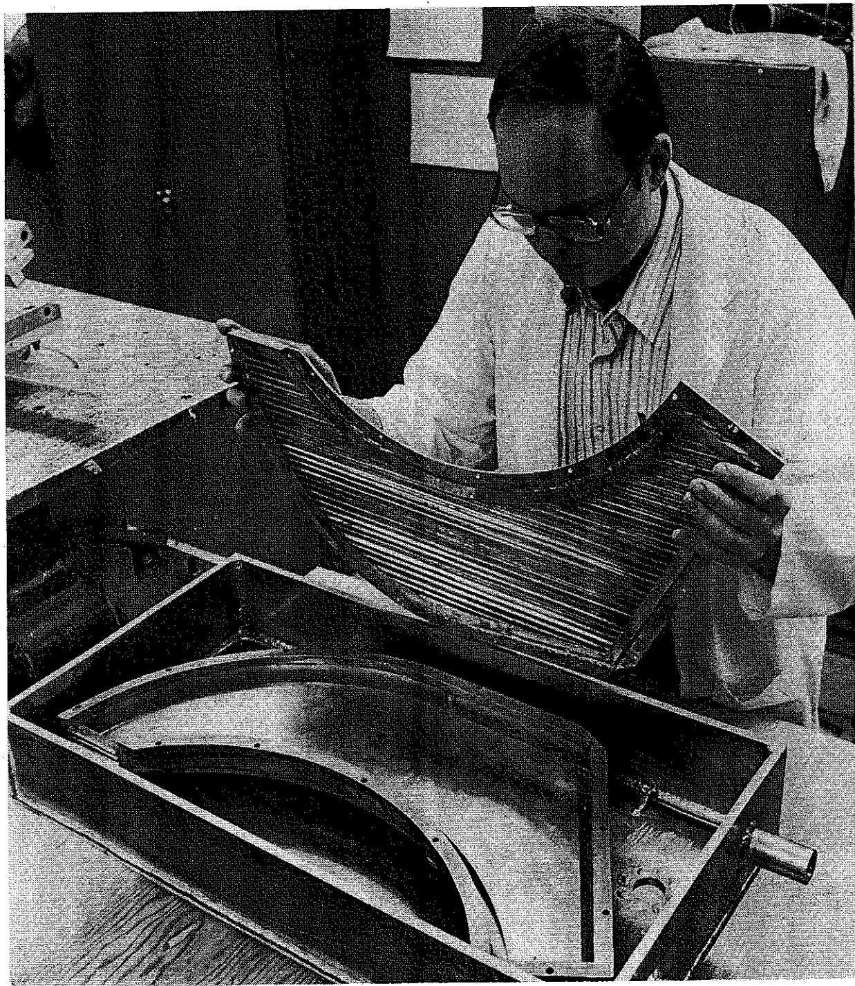
Fig. II. 15. Prototype cryopumping panel being set up for tests in a rectangular dummy aluminum vacuum box. The panel will ultimately mount inside the dee, the outer crescent shaped box in the figure being at 80^{\circ}\text{K} with the chevron in the worker's hand facing the beam space and protecting the 4.5^{\circ}\text{K} surface.
